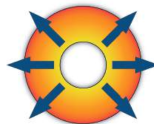
HEATING EXPANDS THE INNER DIAMETER
