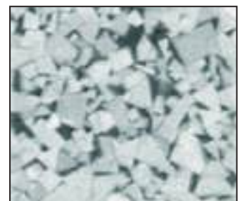
Sub-micrograin carbide 0.5 - 0.9 \mu\text{m}
